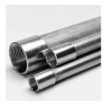
East Electrical hot dip galvanized electrical rigid conduit is manufactured with high-strength steel. Rigid conduit is zinc coated both outside and inside with a hot dip galvanizing process. Produced in normal trade sizes from ½" to 6" in standard lengths of 10ft. Both ends of the pipe are threaded, with a coupling supplied on one end.
